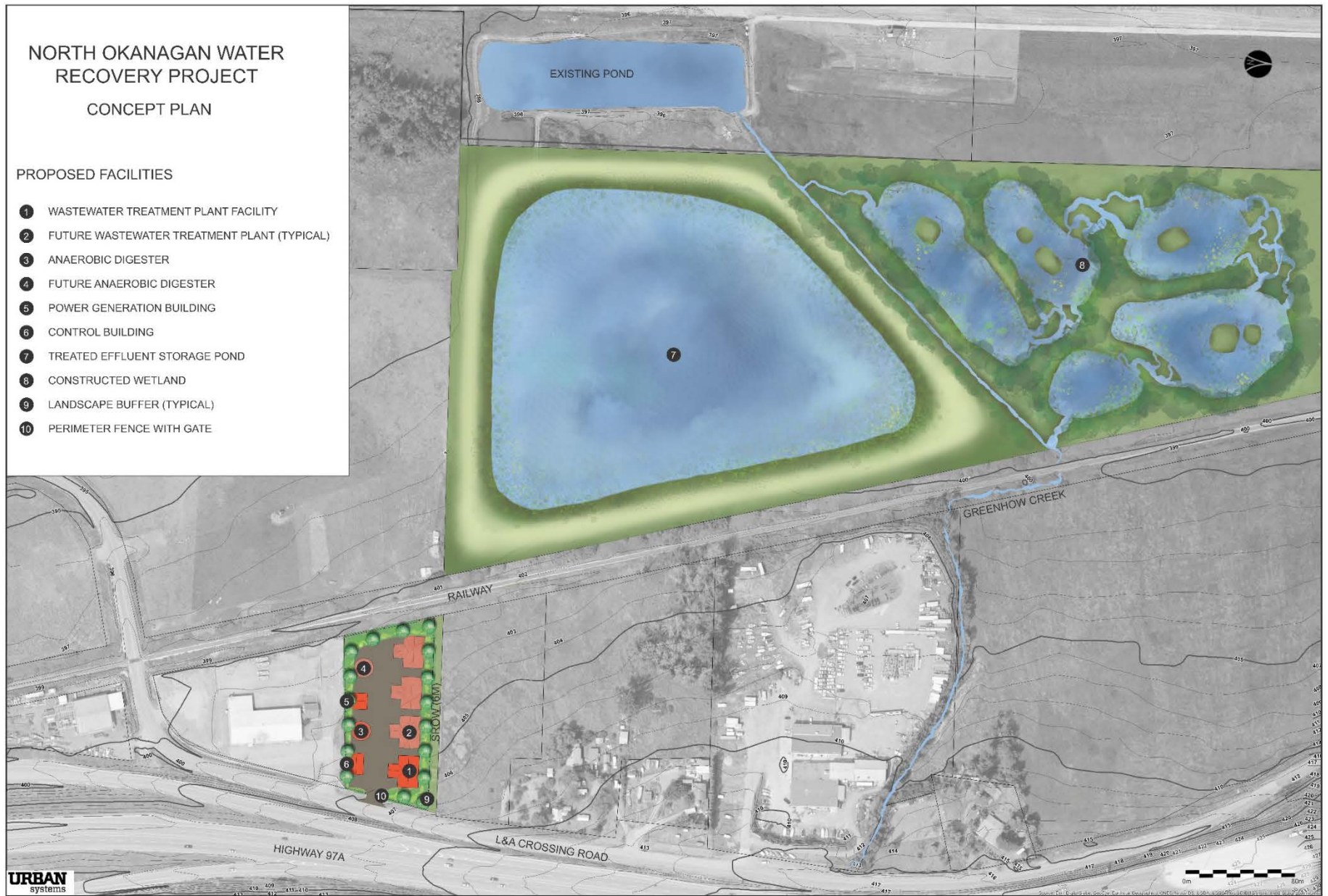
Figure 4.2: Wastewater Recovery System Site Plan
